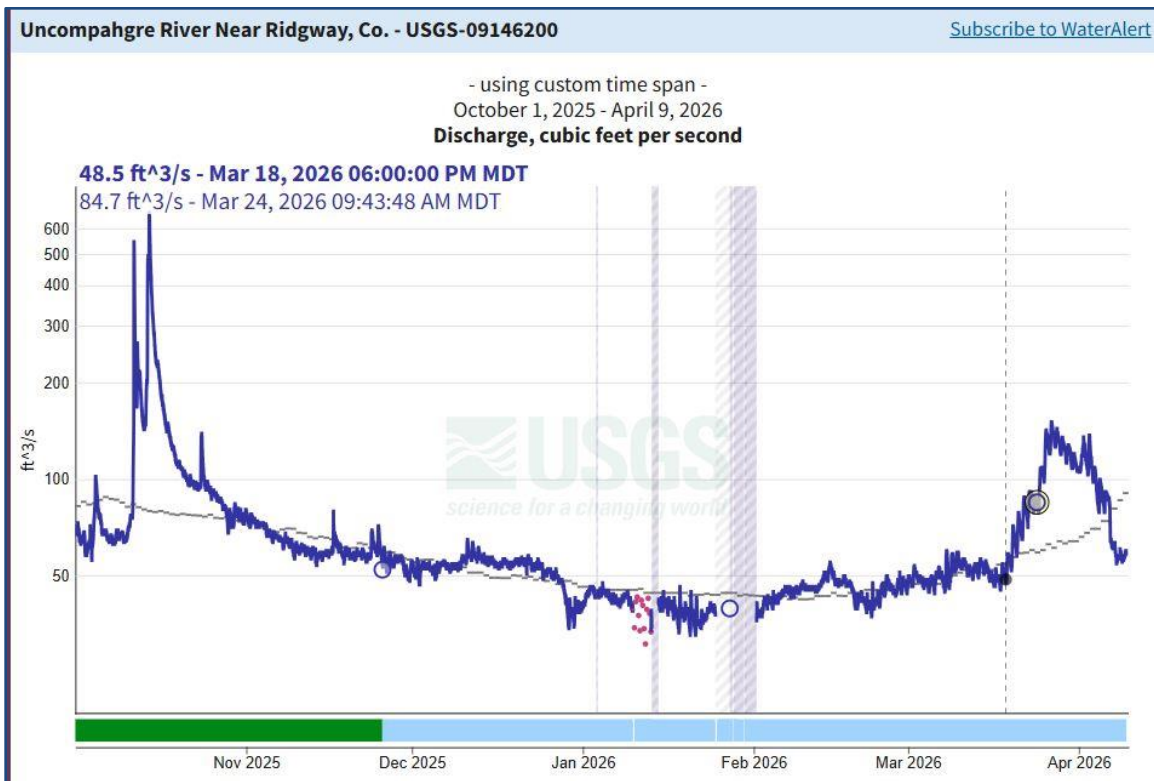
Figure 2. Hydrograph for the USGS gauge near Ridgway, CO, October 1 st , 2025 through April 9 th , 2026. Gray line is the median discharge. Hatched areas are ice affected periods and red dots represent estimated discharge. Vertical dashed line shows date when runoff from snowmelt began on about March 16 th .
